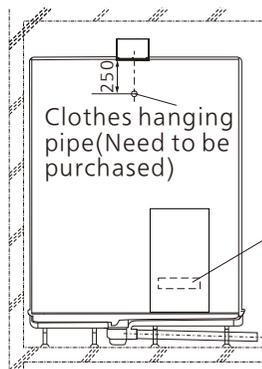
To make the effect of drying clothes better, please set a ventilation shutter at the lower part of the door with a valid opening area of 100 cm<sup>2</sup> or above.
